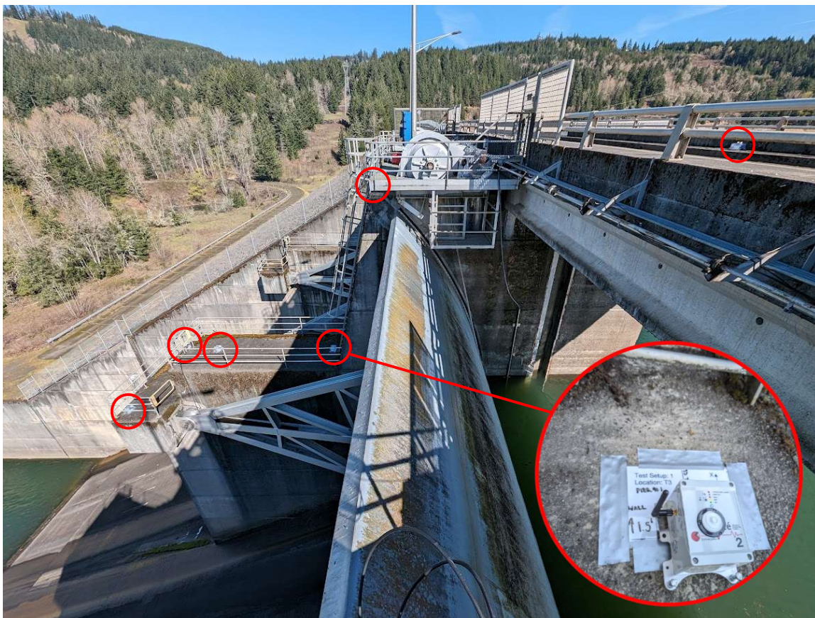
Figure 8. Photo of the Test Setup 2 (TS-2) with emplaced instruments. Inset photo of archetype instrument emplacement with bubble level, location number, sensor number, test setup number, and measurements to local structural reference points.
